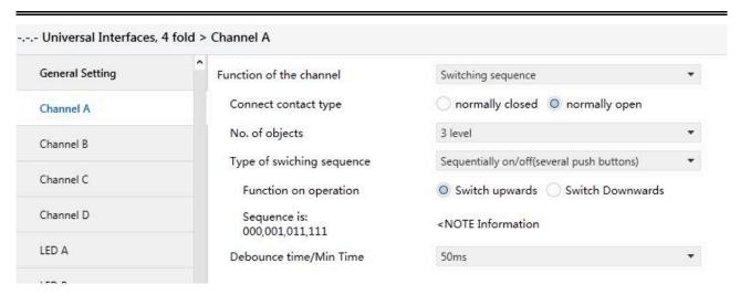
Fig.11 Parameter window "switching sequence, X"
