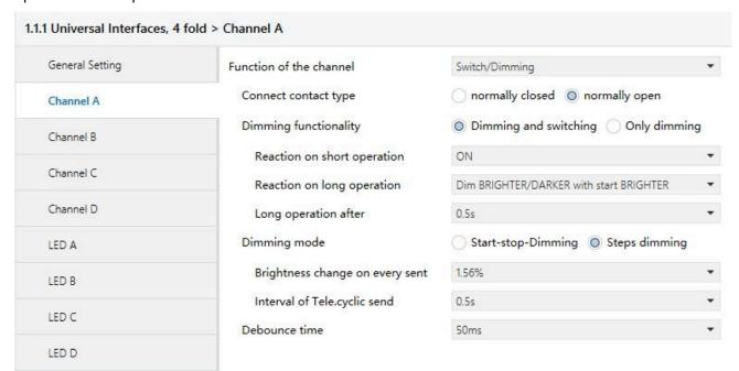
Fig. 5 Parameter window "Switch/Dimming"
