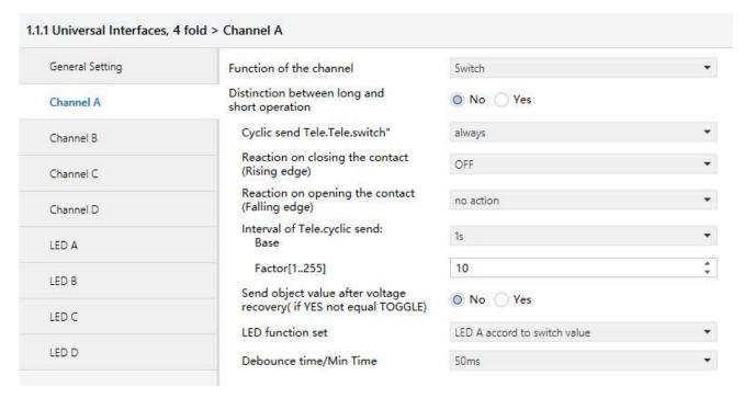
Fig.2 Parameter window "Switch X" (do not distinguish between long and short operation)
