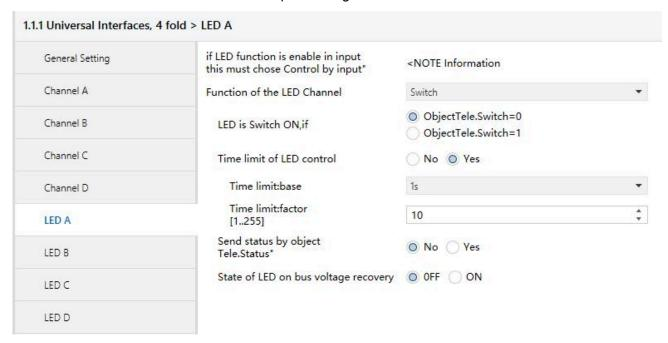
Fig.17 Parameter window "Switch, X"
