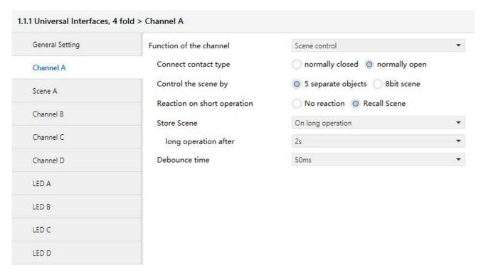
Fig. 8 Parameter window "Scene control, X"
