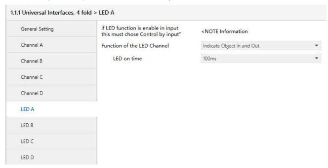
Fig.21 Parameter window "Indicate object in and out, X"
