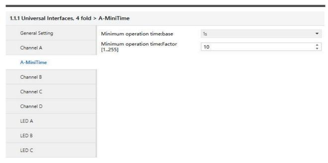
Fig. 3 Parameter window "X-Mini Time"
