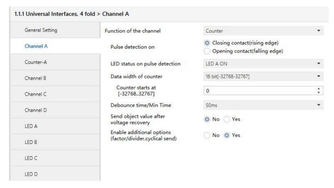
Fig.12 Parameter window "Counter, X"
