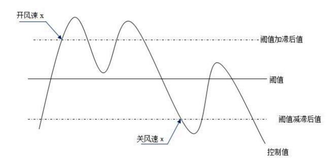
In the case of lag is enabled, if the temperature difference overlap occurs, the action of the fan is treated like the PI control mode.
