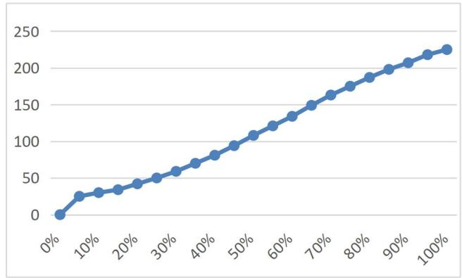
Fig.2: 1.5 exponent dimming curve
