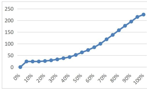
Fig.4: 2.5 exponent dimming curve
